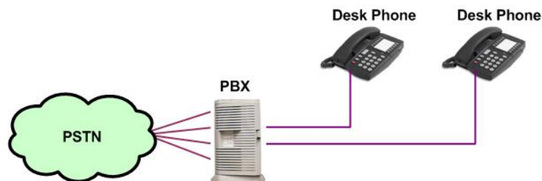
Figure 2: Analogue Telephone Connections (before)
